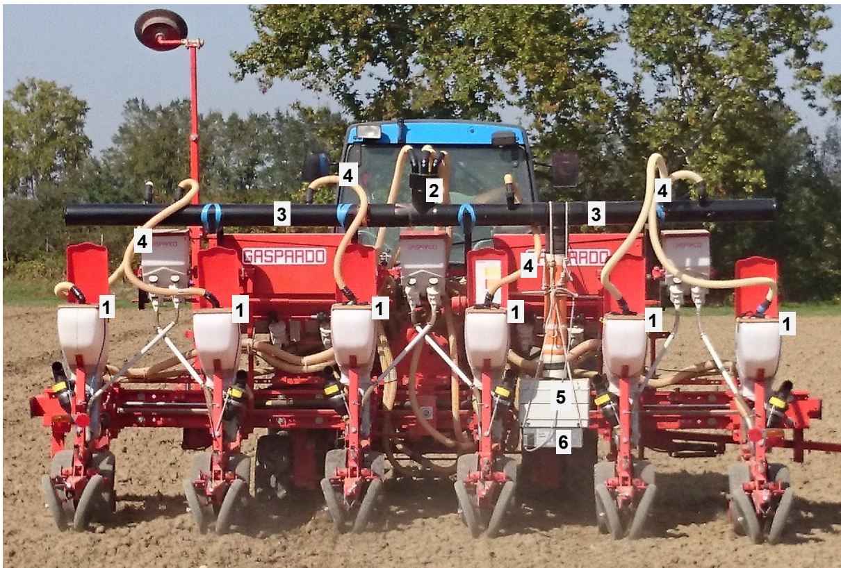
Figure 1. Modified drill with the recycling-filtering device. (1) hoppers' tight lids replacing the normal lids; (2) collector of pipes coming from the drill's fan; (3) main collector pipe; (4) recycling pipes from each hopper to main collector; (5) box containing the anti-pollen filter with activated carbon filter; (6) electrostatic filter and filtered air outlet.
