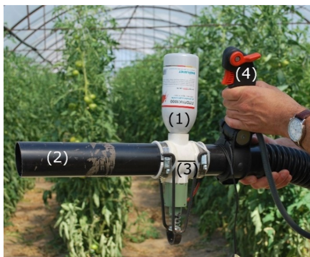
Figure 1. Blower device (Pezzi et al. , 2015), for predatory mites mechanical release. 1) Bottle containing beneficial organisms, 2) air diffuser, 3) extraction system operated by electromagnet for rod frequency regulation, 4) command lever for air speed regulation.
